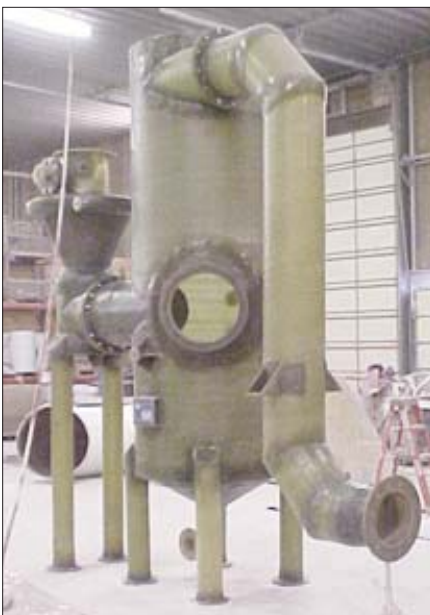
Scrubber, Venturi Type
